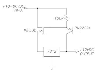
This circuit uses a low input voltage (<40V) regulator like a 7805 or 7812 and puts a high voltage pre-regulator on its input. The PN2222A is connected as a temperature compensated 6.8V zener diode. The "anode" of this zener is connected to the +12V output of the 7812 regulator. This makes the zener "cathode" voltage 18.8VDC. The 100K resistor acts as the zener current limit resistor that connects to the high voltage input.
